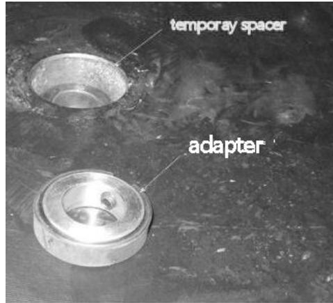
Fastening an adapter to an individual plate. With an adapter fastened to an olympic plate, the plate can be added and removed from the bar as if it was a standard plate.
