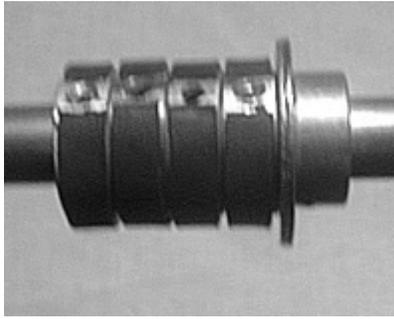
Tightening the adapters to the bar. If you have plate setups with the olympic plates staying in the same position workout to workout, you can set up some adapters in fixed positions by tightening the set screws (use the 5/16" short set screws). Each adapter is 5/8" (.625") thick.
